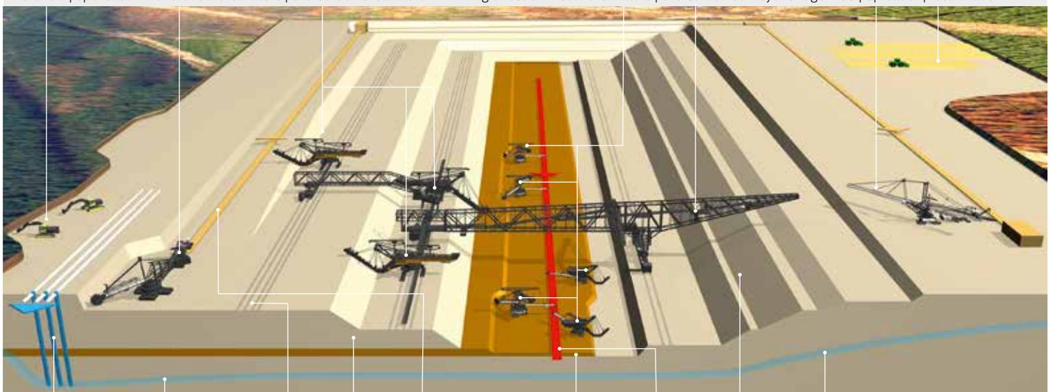
filter well | lowering of groundwater level | tracks | overburden | overburden conveyor belt | lignite | lignite conveyor belt | Dump | rise of groundwater
